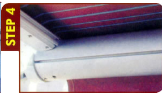
STEP 4 Extend the AntiFlap Kit out and fit the spigot into the hole in the roller
