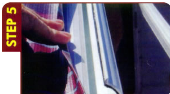
STEP 5 The edge of the awning fabric is now located between the bottom and top clamp sections of the AntiFlap Kit
